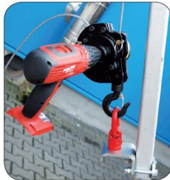
fixed at the tripod, using an adapter plate with stop ring
